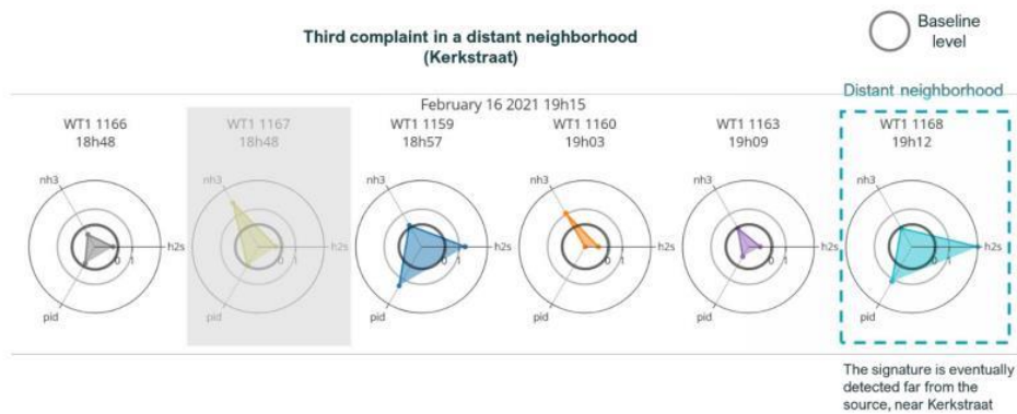
Figure 6 : Gas signature of events recorded on WT-1s before the complaint filled out from Kerkstraat at 19h15.
