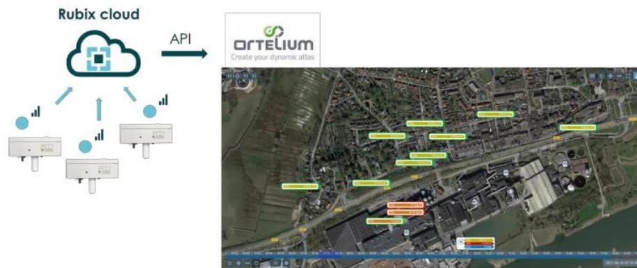
Figure 1 : View of the system setup and Ortelium platform interface showing nine of the ten WT-1 monitoring stations (yellow insets), the three VOC sensors installed near the most southern source of pollution (orange insets), and the wind data feed (blue arrow). Sources of emission are depicted
